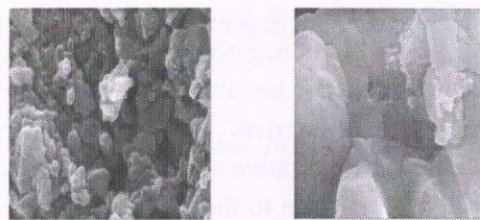
Fig. 2. SEM image of pure CoS 2 and CoS 2 in polymer matrix nanoparticles
